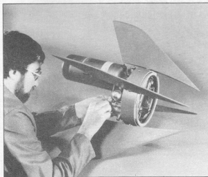
British Aerospace Canard control system for the Penguin Mk 3 missile produced by Kongsberg Vapenfabrikk.
